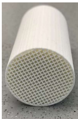
Figure S1 Photograph of the ceramic honeycomb body (Ø 25,4 x 50mm) used as substrate for \text{Na}_2\text{SO}_3 coating in this study.
