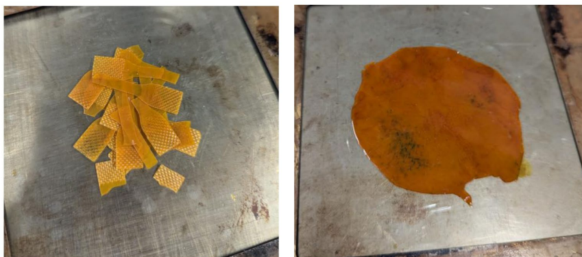
Figure S145: Before and after reprocessing for 1 h at 130°C.
