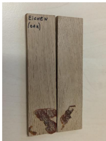
Figure S151: Wood (oak) plate after lap shear measurement, the chunks of wood that remain attached to the polymer suggest a structural type of failure.
