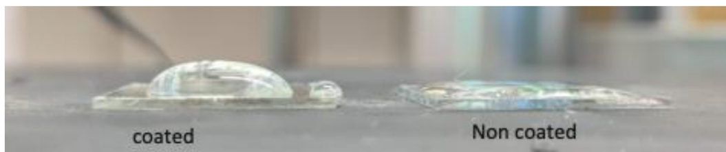
Figure S 74: Water drops on glass slide. The left slide underwent a dip-coating procedure, involving immersion in the cross-linking mixture for a duration of 5 seconds. Subsequently, the coated slide underwent air-drying overnight leading to an increase in hydrophobicity.
