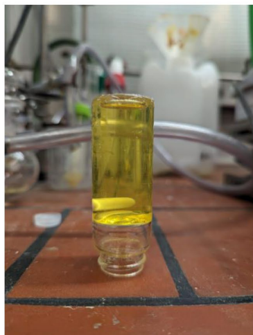
Figure S 67: Vial inversion test of polymerisation mixture after crosslinking.
