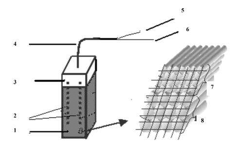
Figure 6. A schematic representation equitensiometer (EQ-15), soil moisture sensor. Labels for components are 1.Equilibrium body, 2. Vertical TDR rods, 3. Soil water content sensor, 4. Cable, 5. Power supply, 6. Signal to logger, 7. Small diameter glass fibres, 8. Large diameter glass fibres.
