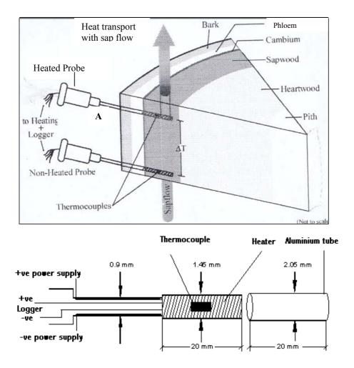
Figure 7. (Above) Schematic representation of sap flow sensor installed on to a tree. The upper probe, labeled A was heated with a constant current power supply while the lower one (reference) was not heated. (Below) Enlarged drawing of the heated probe (A), showing detailed construction and wiring of the sensor. (Courtesy of Ecomatik, Dachau Germany).
