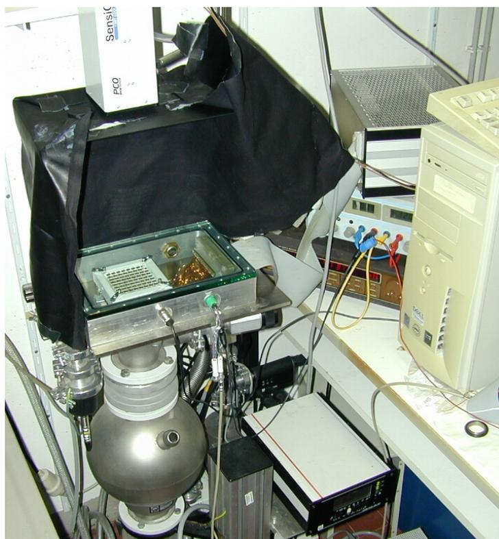
Figure 3.25: *Photograph of the OLED analysis setup: In the foreground the measuring chamber with an OLED device installed, in the background the multiplexer electronic, a power supply and the SMU together with the controller PC.*
