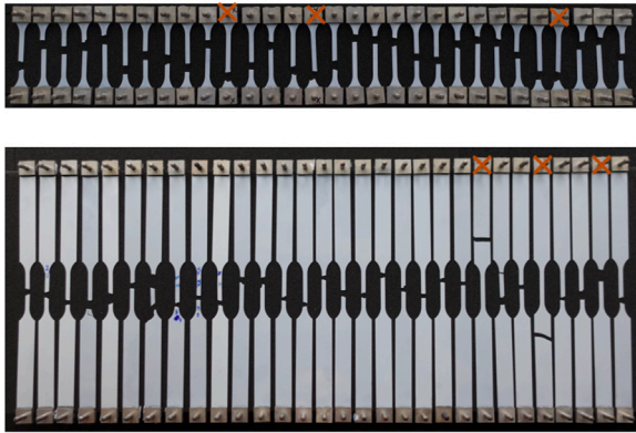
Fig. 3. Overview of the complete set of tested samples. On the top of the picture are positioned the 30 samples tested at room temperature and on the bottom the 30 samples tested at high temperature. The invalid samples are marked with an orange cross. (For interpretation of the references to color in this figure legend, the reader is referred to the web version of this article.)
