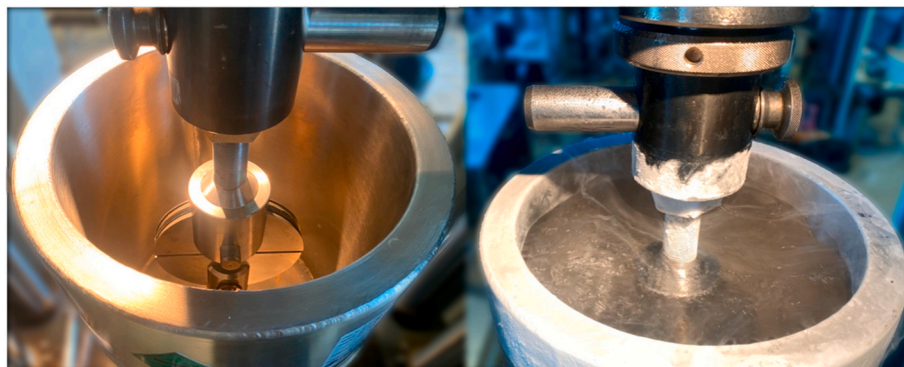
Fig. 3. Schematic NOL-ring tensile in-situ testing setup with LN2.
