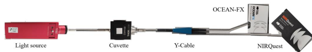
Figure 3. Experimental setup for transmission determination with two spectrometers, OCEAN-FX and NIRQuest.
