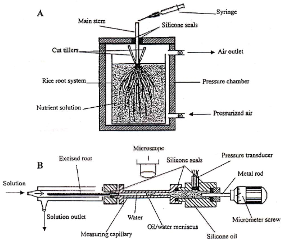
**Fig. 6** Pressure chamber (A) and root pressure probe (B) for measuring water flow across root systems and individual roots of young rice plants. (A) The pressure chamber provided the steady-state water flow across the roots by applying pneumatic pressure to the medium. By using silicone seals, the base of the main tiller was tightly sealed to the pressure chamber. Cut ends of the remaining tillers were clamped and
