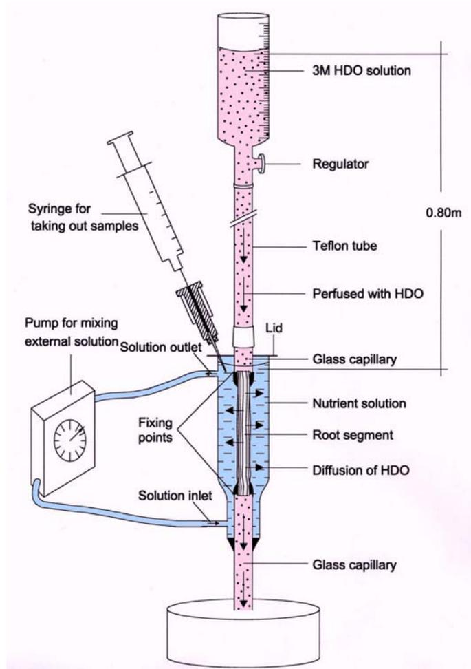
**Fig. 2** Experimental set-up to measure the diffusional water permeability of the outer part of rice roots. Open ends of root segments were fixed to glass capillaries. Aerenchyma within segments was rapidly perfused with 3M heavy water (HDO). At different time intervals, concentration of HDO diffusing into the outer medium was measured with a freezing point osmometer. The external solution was stirred vigorously throughout the experiment, using a small pump.
