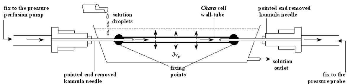
**Figure 2** Pump perfusion set-up: Open ends of cleared *Chara* cell wall preparations (untreated walls or ghosts containing copper ferrocyanide precipitates) were fixed to kannula needles (without pointed end), and inlet ends connected to a Braun-Melsungen pump through a Teflon tube. The pump created pump rates of  $3$  to  $6 \times 10^{-11} \text{ m}^3 \text{ s}^{-1}$ . The other ends (outlet ends) of preparations were connected to a pressure
