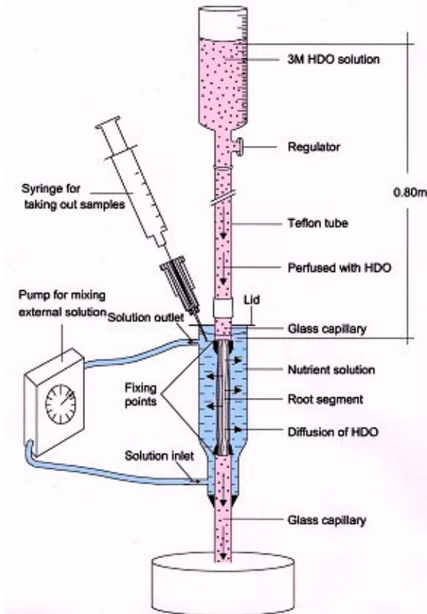
**Fig. 8** Experimental setup to measure the diffusional water permeability of the outer part of rice roots. Open ends of root segments were fixed to glass capillaries. Aerenchyma within segments was rapidly perfused with 3M heavy water (HDO). At different time intervals, 50  $\mu$ l of external solution was taken out using a syringe and concentration of diffused HDO into the outer medium was measured with a freezing point osmometer.
