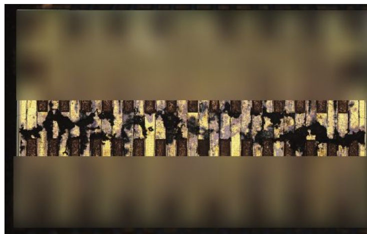
Figure 12. Decapsulation of a GaN dMode device.
