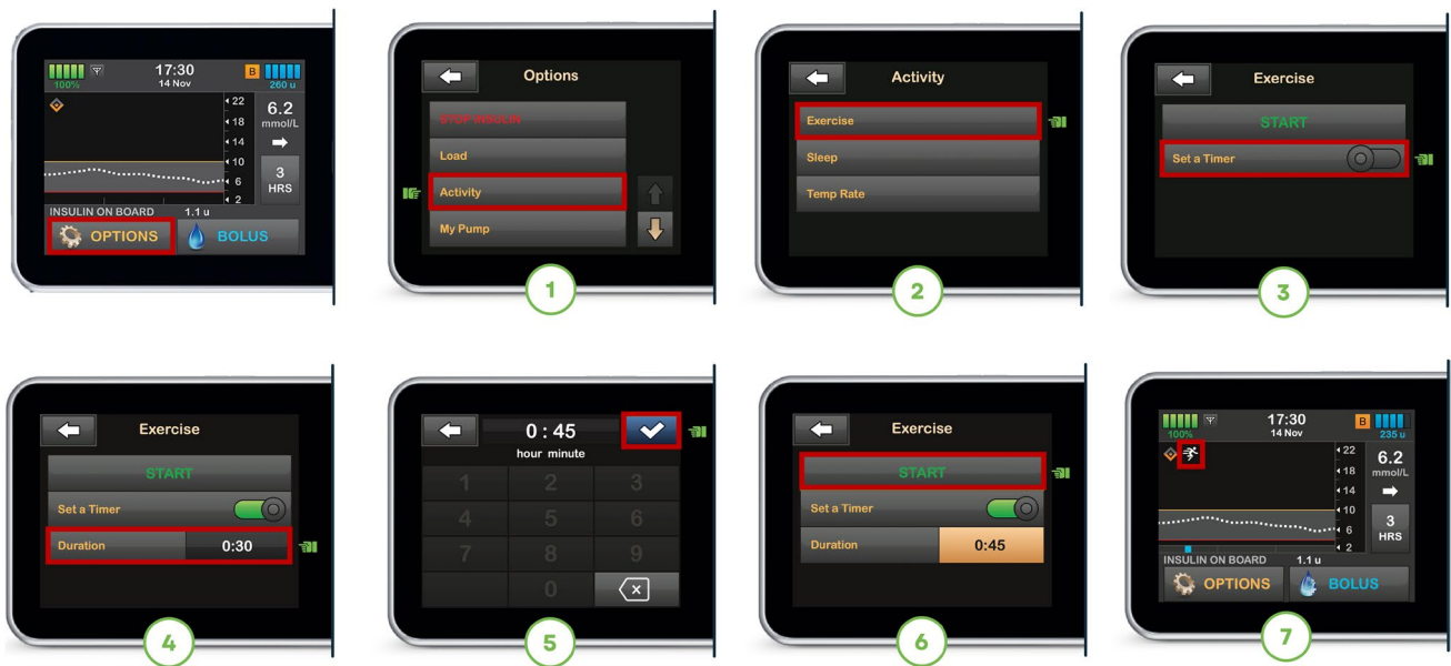
Fig. 11 Illustration of how to set the Exercise mode on the t:slim X2 Control-IQ system. See ESM 1 for version of this figure with glucose concentrations in mg/dl. This figure is available as part of a downloadable slideset
