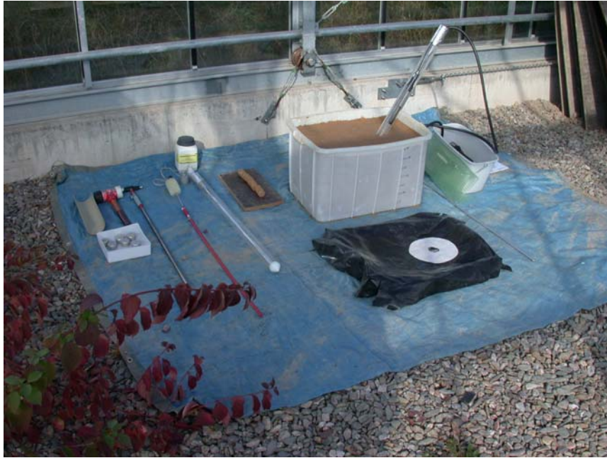
Figure 13 Reference box filled with subsoil for assessment of conversion factors between volumetric soil moisture measured with trime RS44 tube probe and gravimetric soil moisture
