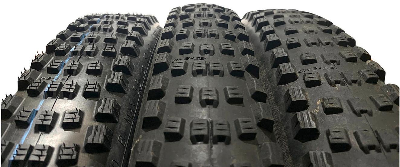
Fig. 3. Comparison between a new, unused tire (left) and a front (middle) and rear (right) tire after a travelled distance of 1500 km.
