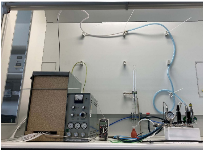
Figure 8. Photograph of the complete measurement setup with furnace, short gas supply line through furnace ceiling, mass flow controllers, and compressed air supply.
