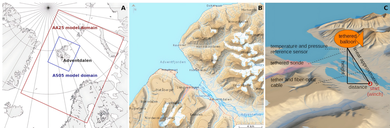
Figure 1. (a) Model domains of the two HARMONIE-AROME numerical simulations (AA25 and AS05) discussed in the present study. Note, that the domain of AS05 was changed compared to the previous study Valkonen et al. (2020). (b) Adventdalen and Adventfjorden ( https://toposvalbard.npolar.no/ , Norwegian Polar Institute). (c) Measurement setup (not to scale) for the tethered balloon carrying the fiber-optic cable and station location (red circle) with three-dimensional topography ( https://toposvalbard.npolar.no/ , Norwegian Polar Institute).
