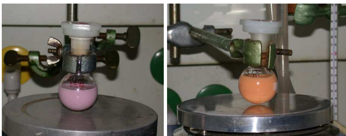
FIG. 5.14. Colloidal ethanolic solutions of the dyes and TiO 2 under stirring. The left picture corresponds to N719, the right one to Ru-TPA 2 .
