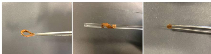
Fig. S25. Pure polyimide membranes (PIM_420), after heat treatment to remove the auxiliary polymer PVP, exposed to different bending states. They include folding, twisting and curling and indicate good flexibility and mechanical stability of the membranes.
