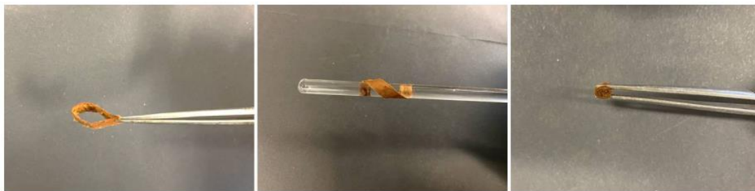
Figure 2-12. The PIM_420 fiber membranes exposed to different bending states. They include folding, twisting and curling and indicate good flexibility and mechanical stability of the membranes.
