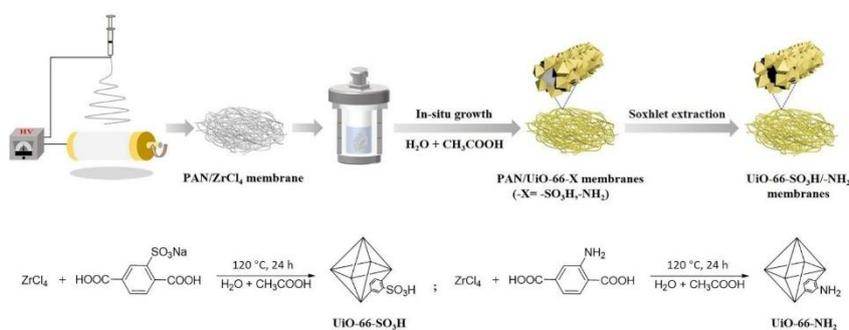
**Figure 1.** Strategy to fabricate the self-standing UiO-66-SO<sub>3</sub>H and UiO-66-NH<sub>2</sub> membranes (top) and the reaction scheme to prepare corresponding MOFs (bottom).
