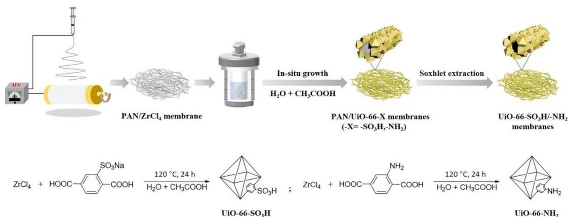
**Figure 2-5.** The template-assisted procedure to fabricate the self-standing 2D MOF membranes: UiO-66- $\text{SO}_3\text{H}$  and UiO-66- $\text{NH}_2$  (top) and the reaction scheme to prepare corresponding MOFs (bottom).
