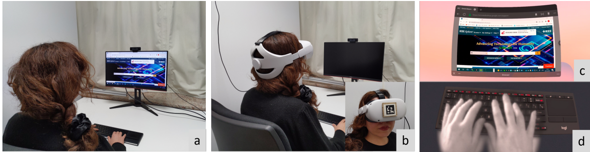
Fig. 1. a) Participant working in a physical desktop setup in one of three physical locations (Germany), including a curved display and a keyboard with integrated touchpad. b) Participant working in the VR setup wearing an Oculus Quest 2, using the same keyboard but a virtual curved display. c) Participant's view within VR where the streamed content from a remote machine is visible. d) Participant's view of the keyboard and hands within VR.
