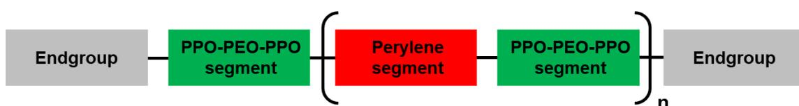
**Figure 34:** Schematic structure of the (AB)<sub>n</sub> segmented copolymers, consisting of repeating units of perylene and PPO-PEG-PPO segments, but show telechelic perylene anhydride groups.
