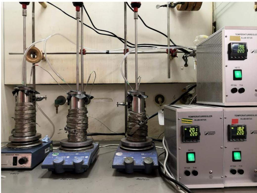
**Figure 27:** Series of three metal reactors used for parallel melt polycondensation reactions for the synthesis of  $(AB)_n$  segmented copolymers out of perylene and selected Jeffamines.
