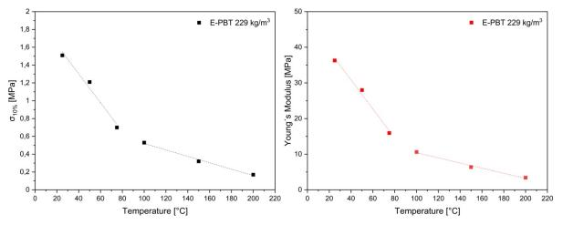
**FIGURE 3:** Temperature dependency of the stress at strain (10%) and the Young's modulus of E-PBT taken from the compression tests.
