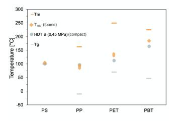
FIGURE 5: Thermal data ( $T_g$  and  $T_m$ ) as well as heat deflection temperature (HDT/0.45 MPa) extracted from data sheets as well as the  $T_{HS}$  measured with the described approach (data partially taken from Himmelsbach et al. [10]).
