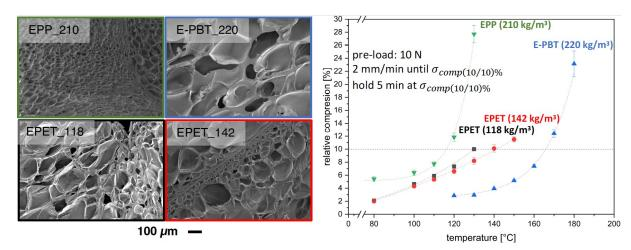
FIGURE 4: Left: SEM images of the investigated foam structures. Right: Relative compression during the creep test at different temperature steps
