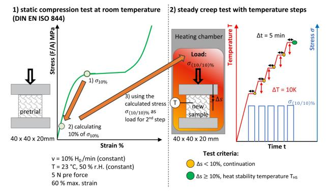
FIGURE 1: Scheme of the measurement principle. In a first step (left) compression test according to DIN EN ISO 844 are carried out to determine a very low load ( $\sigma_{(10/10)\%}$ ), which is applied in the second step (right) – a creep test with temperature steps. (image by Himmelsbach et al. [10], used under CC BY 4.0)
