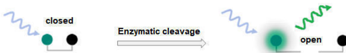
Figure 11. Schematic representation of an assay for the enzymatic cleavage of a doubly-labelled fluorogenic probe equipped with fluorescent reporter (green circle) and fluorescence quencher (black circle) [picture freely modified from Kempf et al. 50 ].
