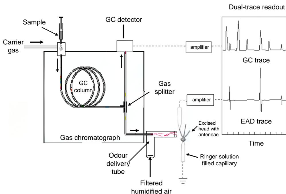
Figure 2. Simultaneous recordings of signals from a FID detector and an insect antenna (EAD). Modified from: [http://www.srs.fs.usda.gov/4501/what\\_is\\_gc.htm](http://www.srs.fs.usda.gov/4501/what_is_gc.htm).
