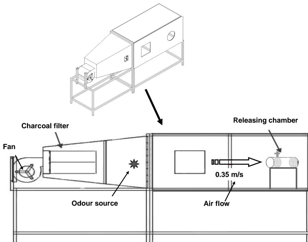
Figure 1. Schematic representation of wind tunnel used for bioassays.
