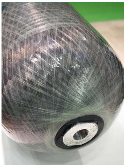
■ Fig. 10: Stable even under very high pressures: hydrogen tank for fuel cell vehicles (sst).
