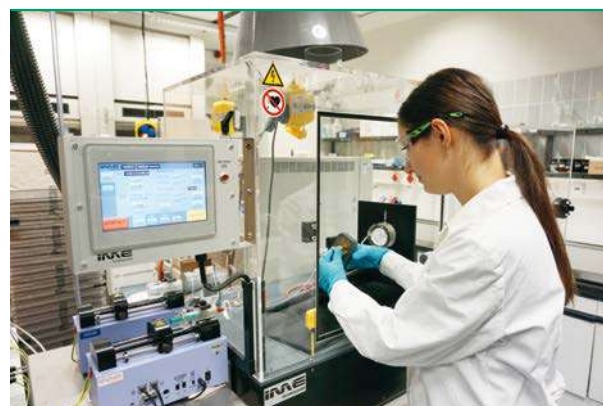
■ Fig. 8: Principle sketch of the electrospinning process (left). Dr. Özner Delikaya prepares a syringe of the polymer solution and places it in the holder (right) (Picture credits: Özner Delikaya, published in her dissertation, FU Berlin).
