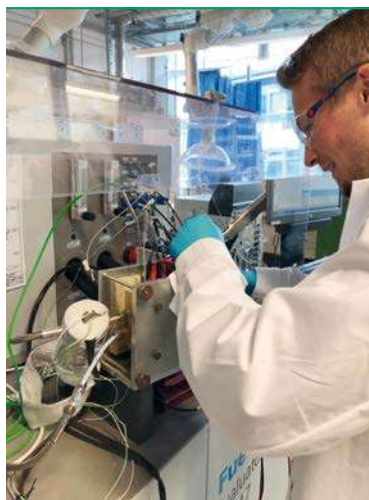
■ Fig. 3 (left): Preparation of a PEMFC test. A membrane electrode assembly with composite membrane is inserted into the measuring cell (Photo: Andreas Rosin).
