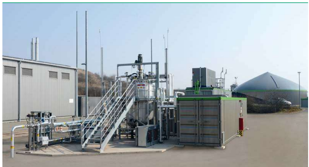
■ Fig. 3: Power-to-gas plant with biological methanation in Allendorf/Hessen. In the electrolyzer, excess electricity is converted into hydrogen (Photo: Viessmann Werke).
