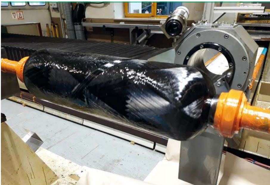
■ Fig. 5 (above): CFRP laminate structure of an ultra-light hydrogen tank concept: 12 individual layers are visible, layered in different directions to fully exploit maximal material performance. Here a reference to aircraft structural laminates becomes visible, where layers at \pm 45 degrees / 0 degrees / 90 degrees / 90 degrees / 0 \pm 45 degrees each result in a quasi-isotropic layered construction (Photo: Fabian Hübner).
