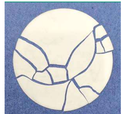
■ Fig. 6: Failed electrolyte sample made of ZrO_2 ( \varnothing 24 mm) (Photo: Tom Liensdorf).
