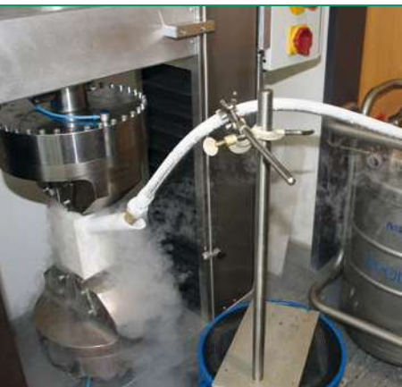
■ Fig. 2: For cryogenic tensile tests of high-strength fibre-plastic composites such as those used for hydrogen tanks, machine forces of more than five tonnes at temperatures of about minus 200 degrees Celsius are required (Photo: Christian Wißler).
