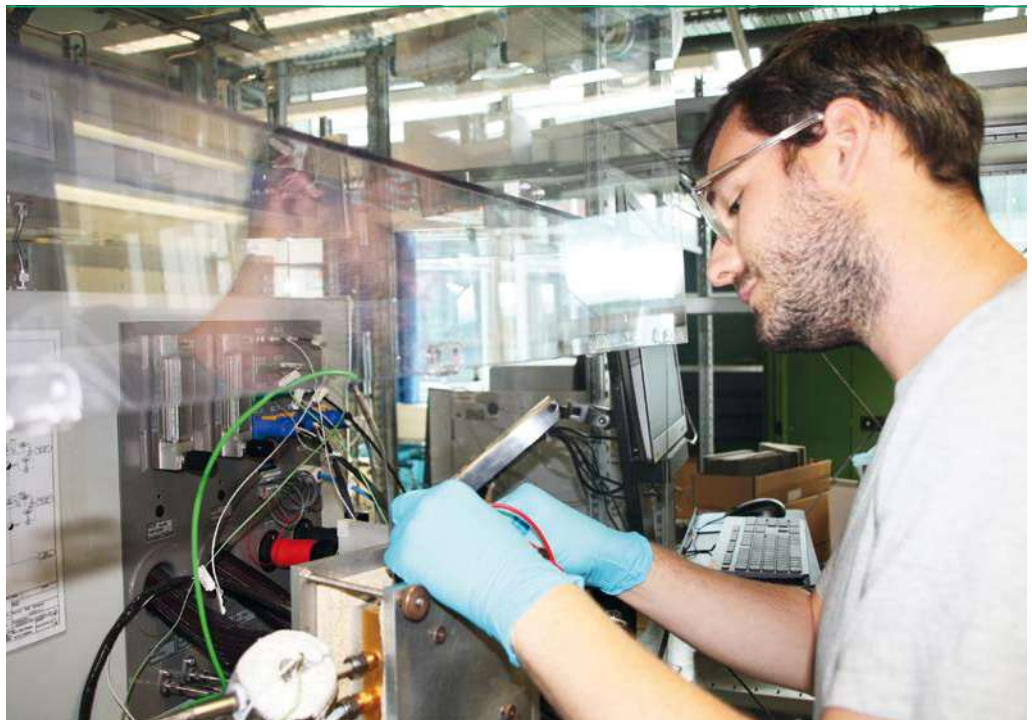
■ Fig. 3 and 4 (Center above): Maximilian Kutter M.Sc. installing a single fuel cell in a fuel cell test bench. With this set-up, specific components such as modified electrodes can be tested on their influence in the fuel cell system (Photos: Christian Wiffler).
