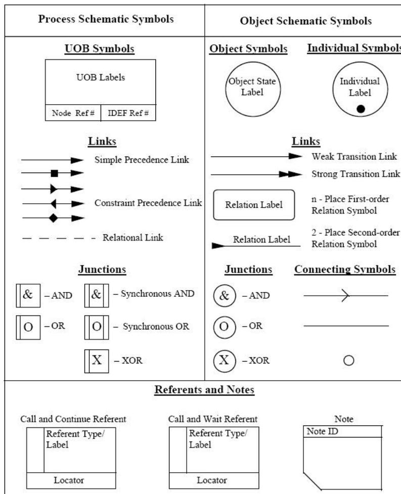
Figure 2.5: Subset of IDEF3 process description schematics
