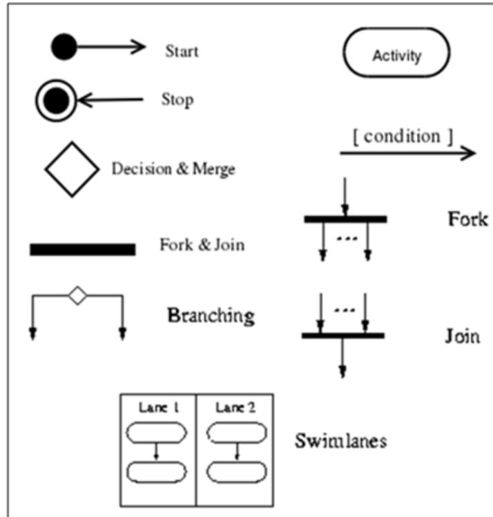
Figure 2.2: Subset of UML AD notations
