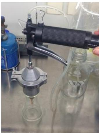
**Figure 5.21:** Photograph of the testing procedure to evaluate the efficiency of prepared filter units to remove *E. coli* from water.
