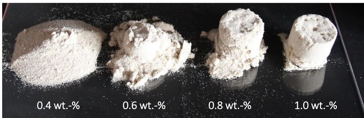
**Figure 5.19:** Photograph combinations of supramolecular nanofibers and sand prepared with different BTA concentrations in the immersion solutions: 0.4 wt.-%, 0.6 wt.-%, 0.8 wt.-%, 1.0 wt.-%. Preparation parameters: Solvent: 2-butanone, Immersion temperature: 50 °C, Cooling temperature: -78 °C, Cooling time: 30 min, Non-solvent: water, Total mass of granulate material: 25 g.
