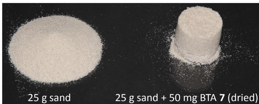
**Figure 5.7:** Photograph of 25 g of sea sand and a sand bed with supramolecular fibers consisting of 25 g of sand and about 50 mg BTA **7** demonstrating the dimensional stability of the prepared samples. Preparation parameters: Solvent: 2-butanone, BTA concentration: 1.0 wt.-%, immersion temperature: 50 °C, cooling temperature: -78 °C, cooling time: 30 min, non-solvent: water, total mass of granulate material: 25 g.
