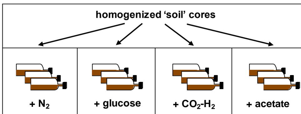
**Figure 11: Experimental set-up of anoxic slurries with 'soils' from contrasting mires.**
