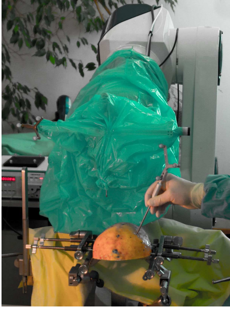
Figure 5.13: User demonstrating the skull surface with an optical tracking pointer, used for both surface sampling or robot scan path definition.
