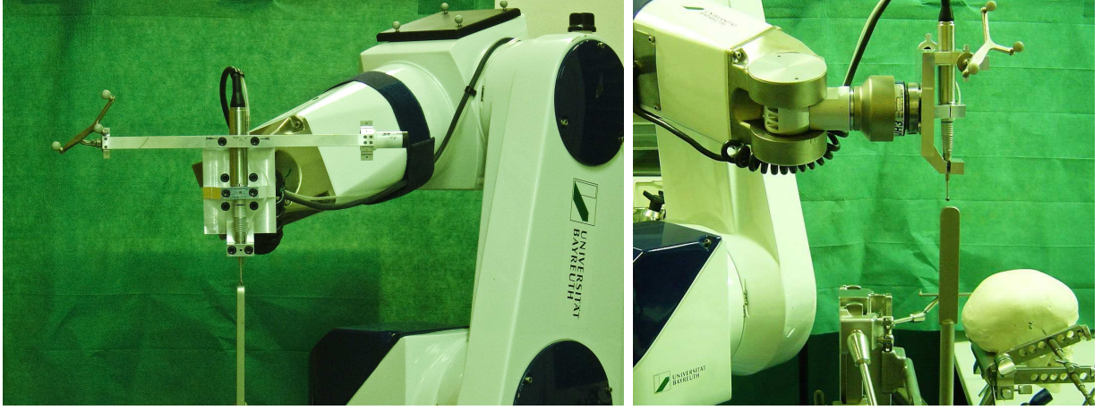
Figure 5.24: Tool calibration setup, with robot-held tool approaching the calibration post.
