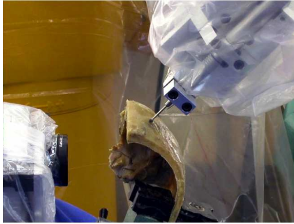
Figure 6.8: Experiment setup for comparison of constant-speed vs. force-controlled milling strategies. An IR temperature camera is aimed at the intervention region from below the skull preparation, as direct measurement of temperatures next to the miller tip is not possible due to the irrigation process.
