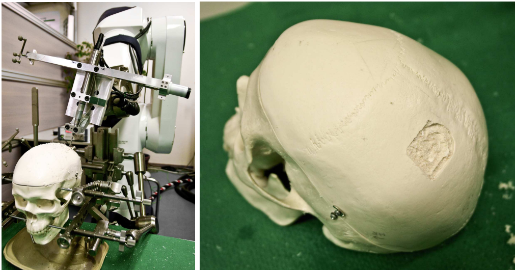
Figure 6.13: Robot-based milling of a generic implant bed for the Combi40+ geometry model (top left) based on a 3D ultrasound map (performed with the CASPAR/RX90 robot) in a synthetic skull dummy. Although the implant cavity is well-aligned with the upper skull surface and does not exhibit any breakthrough into the skull interior, milling in the plastic material produces detritus in the cavity making objective quality assessment and implant insertion difficult.
