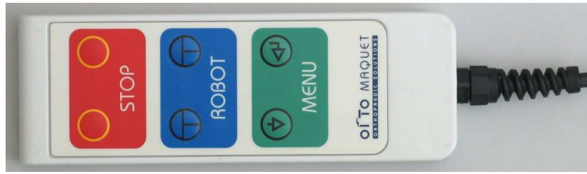
Figure A.2: Manual control pendant connected to the robot controller. The two redundant STOP buttons (red) are hardwired into the controller emergency shutdown circuit, while the two redundant ROBOT buttons (blue) and the MENU buttons can be queried by robot controller programs in software.
