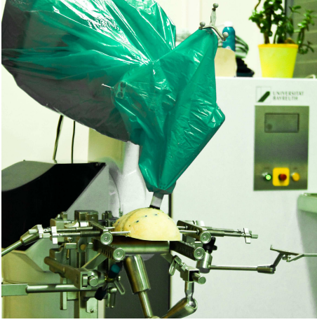
Figure 5.17: Robot-based ultrasound scan. The ultrasound probe is guided perpendicularly along the skull surface under force-based pressure control.
