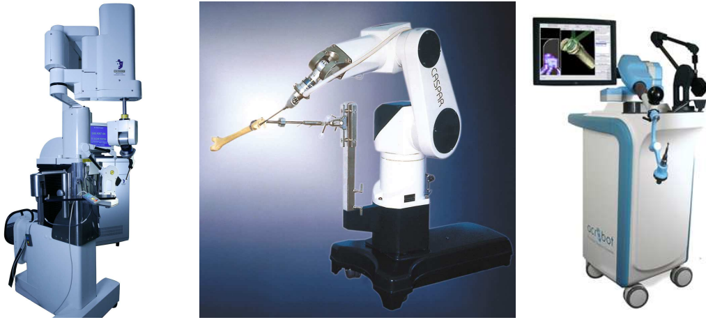
Figure 1.3: Orthopedic robot systems: Autonomous systems ROBODOC (IBM / Integrated Surgical Systems Inc., now part of Curexo Technology Corporation/ www.robodoc.com ) and CASPAR (former Orto-Maquet GmbH), cooperative system Acrobot/Sculptor (Acrobot Co., now part of Stanmore Implants Worldwide, Ltd.) (from left to right).
