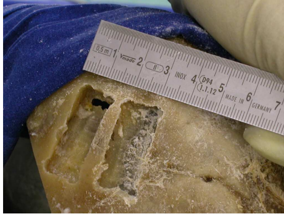
Figure 6.11: Dummy volumes from robot-based milling in a human skull preparation with an early system version (based on the RX130 setup). With constant-speed miller feed (without speed control), the variations in forces led to highly imprecise results, visible in particular along the outer ridge, where irregular chips broke off the bone surface. Also, it is apparent that force-following three-point registration is not sufficient to define a milling volume that does not cause breakthroughs into the skull interior (left volume).
