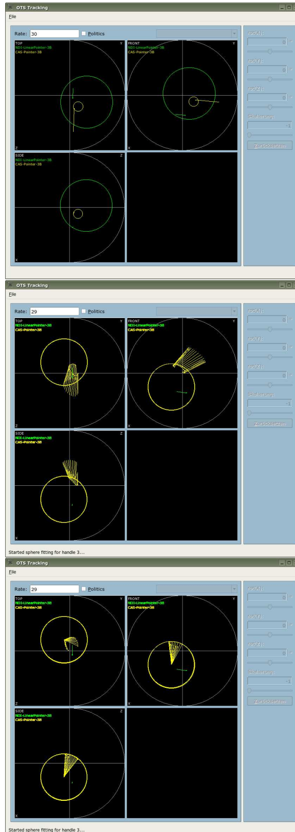
Figure 5.30: Pointer calibration by means of sphere fitting during pivoting. The uncalibrated pointers are moved into the OTS workspace, when fitting starts (top). When the estimated pivot center point stays stable long enough, collection of the sphere centers begins (center). When a certain time threshold is reached without disturbance of the centers, the calibration is completed (bottom).
