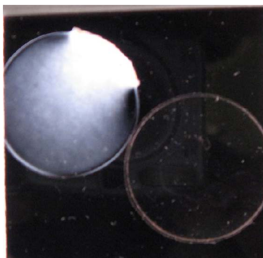
Figure 4.57: Images between crossed polarizers of injection molded samples of PMMA 7H before ( left ) and after ( right ) the annealing process (20 h at 135-140 °C under vacuum).
