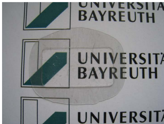
Figure 4.54: Image of a thick film (1.5 mm) of a blend of PMMA (7H) with 1.5 wt% of diblock copolymer 4c prepared in hot press.
