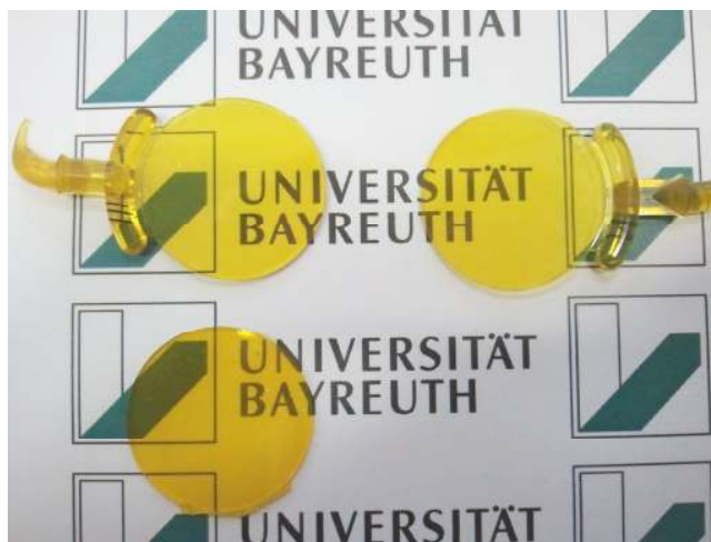
Figure 4.56: Images of the injection molded samples: PMMA (7H) with 0.75 wt% ( top left ) and 1.5 wt% ( bottom left ) of methoxy azobenzene-containing diblock copolymer 6b as well as PS (165 H) with 0.75 wt% methoxy azobenzene-containing diblock copolymer 12a ( top right ) prepared by powder-powder mixtures.
