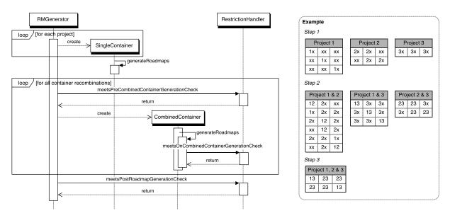
Figure 2. Roadmap Generation and Restriction Handling
