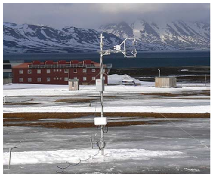
Abb. 2: Turbulenzmesskomplex in Ny-Ålesund, Spitzbergen, 79° N (Foto: Lüers)
