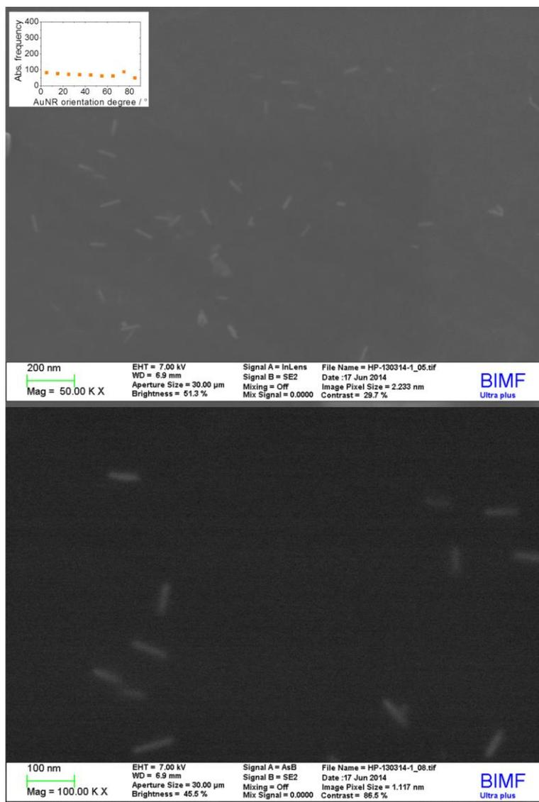
**Figure 7.S8.** SEM micrographs of AuNR@TISIT embedded in Kraton FG1901x at 0% elongation, including the corresponding OD function.
