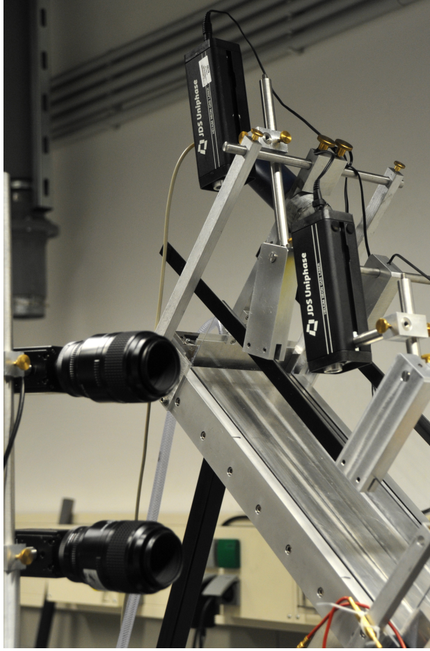
Figure 2.11: Photo of the experimental setup for the measurements of the free surface stability.
