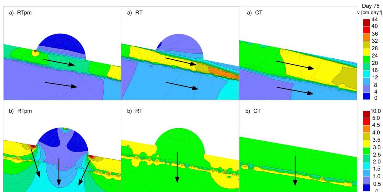
**Fig. 8.** Flow velocity during a monsoon event (day 75) under different management systems at field site 1 and field site 2, black arrows indicate the main flow direction.
