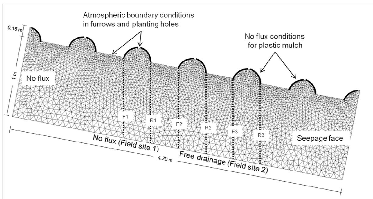
**Fig. 4.** Boundary conditions of the model simulations; note that the bottom boundary varies between the two field sites; vertical meshlines F1-3 and R1-3 were included to calculate lateral water fluxes (see Fig.9); for simulation of ridges without coverage (RT) and conventional tillage (CT) atmospheric boundary conditions were implemented at the entire surface.
