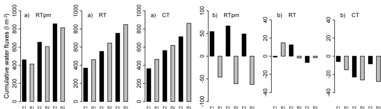
**Fig. 9.** Cumulative water fluxes at the transition from furrows to ridges (F1-3) and from ridges to furrows (R1-3) in slope direction, see also the graphical implementation in Fig.4. Due to different bottom boundary conditions at both field sites, only positive cumulative water fluxes are simulated at field site 1 due to mainly lateral water movement, at field site 2 the main vertical water movement results in positive and negative water fluxes; a) field site 1, b) field site 2
