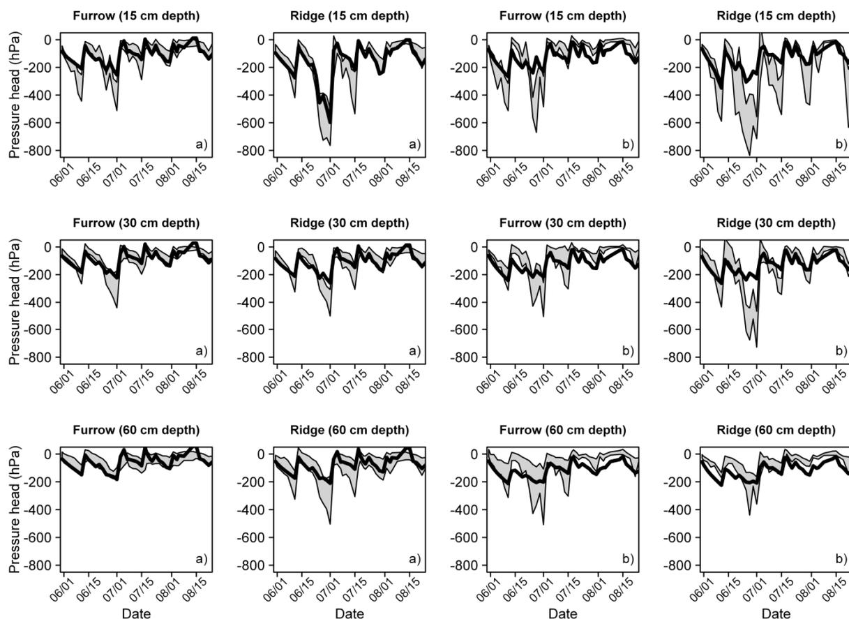
**Fig. 5.** Observed vs. simulated pressure heads at different depth for a) Field site 1 and b) Field site 2; limits of grey area =  $\pm$  standard deviation of the observed data, black solid line = simulated pressure heads.
