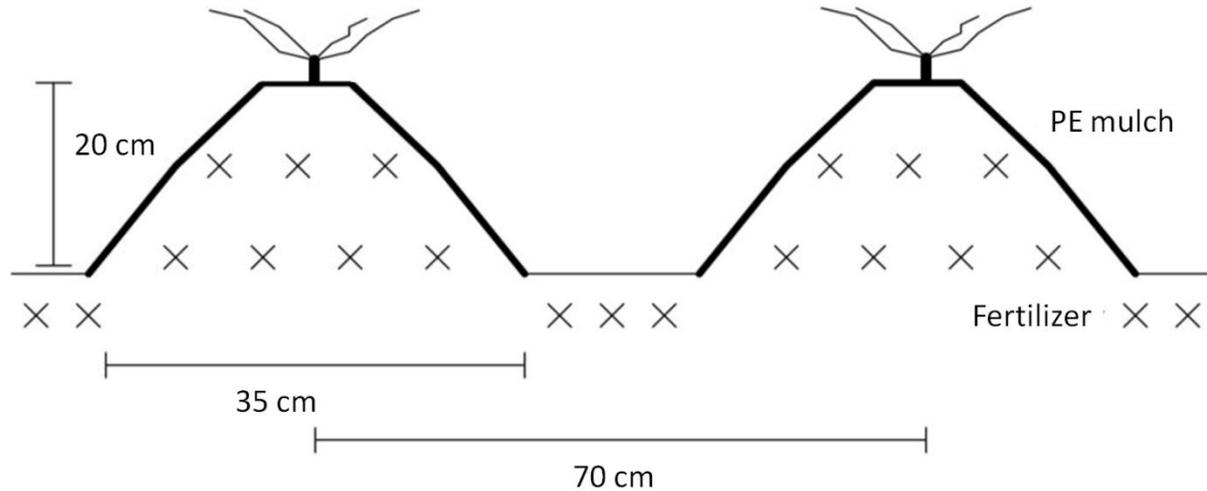
**Figure 2.2** Scheme of a typical ridge cultivation system with plastic mulching in a temperate South Korean area with summer monsoon. Shown are the distributions of N fertilizer in the system and width, height and distance of the ridges
