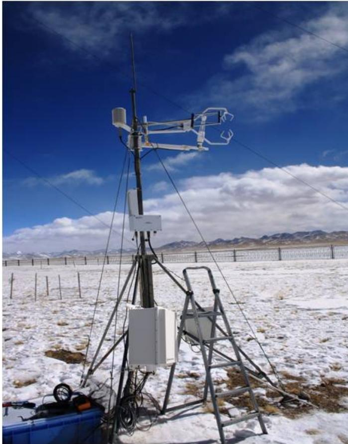
**Fig. 1.** Eddy-covariance station with the CSAT3, Li-7500, KH20 and HMP45 at NAMORS in February 2010.
