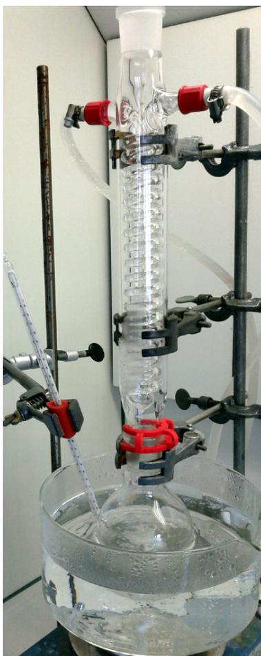
Figure 2.3: Experimental setup used to prepare the sol.
