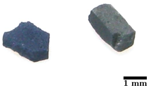
Figure 5.5: Fragments of sintered pellets of samples gel3-3 (left) and gel3-2 (right) synthesised at  $\log f_{\text{O}_2} = -11$  and  $\log f_{\text{O}_2} = -16$ , respectively. The former sample is blue due to the presence of the  $\text{Ti}^{3+}$ - $\text{Ti}^{4+}$  pair while the latter is greyish, likely due to colourless hibonite (appearing white in the bulk sample) with minor quantities of dark blue/black corundum containing traces amounts of  $\text{Ti}^{3+}$ .
