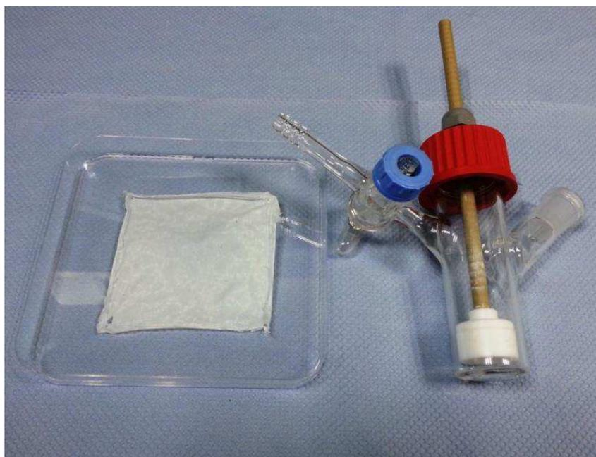
**Figure 5.8.** The tube material (white square, ca.  $7 \times 7$  cm) was folded and placed inside the white Teflon chamber of the custom made sample mount (right).
