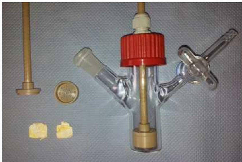
**Figure 4.8.** Special apparatus used for the functionalization of the nanotubes and the catalytic cycles.
