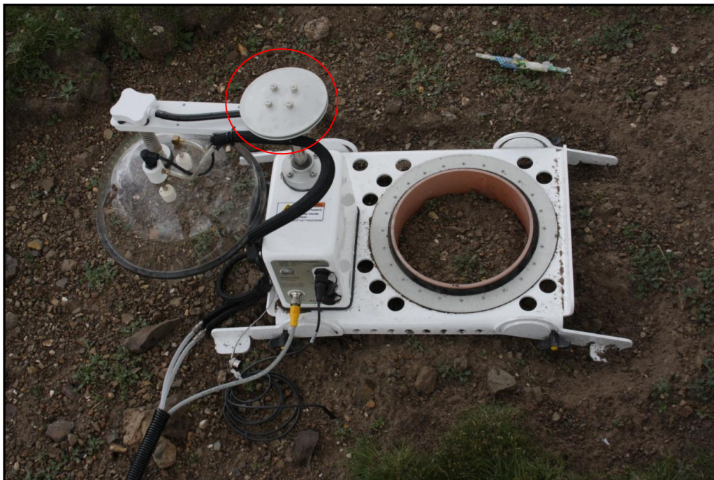
Fig. 5-1: Li-COR Long term CO 2 flux chamber for measuring the net ecosystem exchange. Red circle indicates the venting tube
