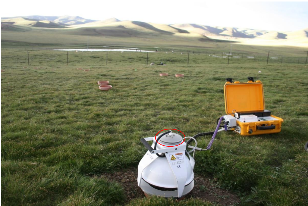
Fig. 5-2: Li-COR Long term CO 2 flux chamber for measuring ecosystem respiration. Red circle indicates the venting tube
