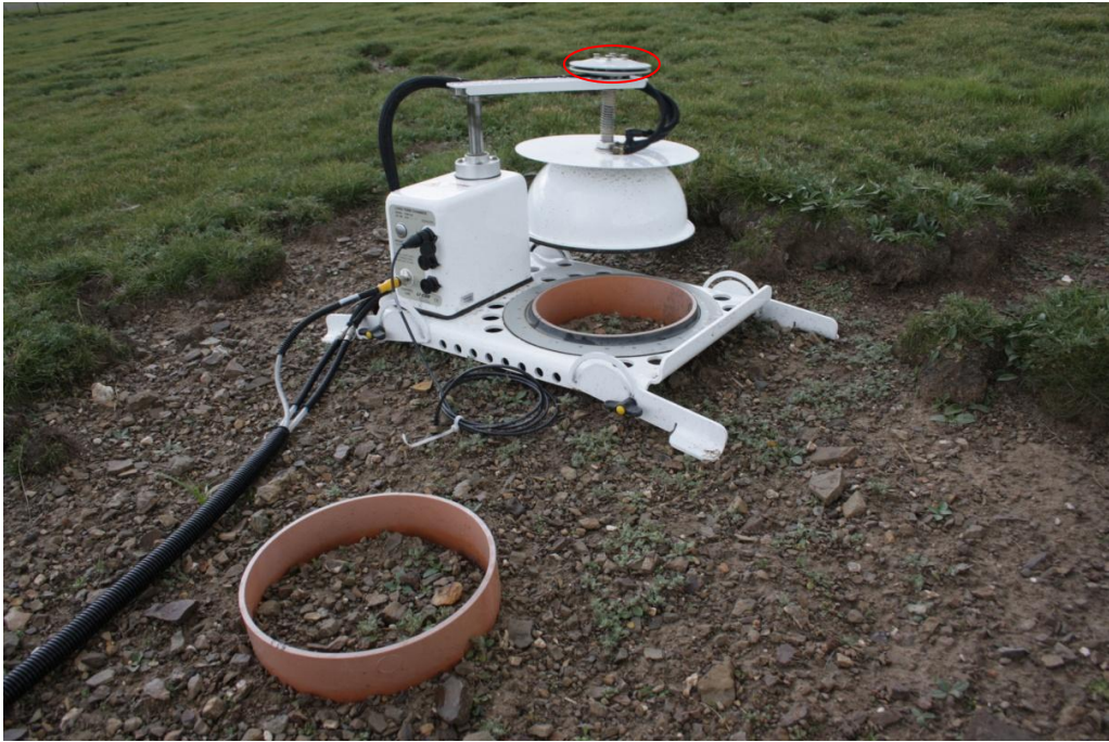
Fig. 5-2: Li-COR Long term CO 2 flux chamber for measuring ecosystem respiration. Red circle indicates the venting tube
