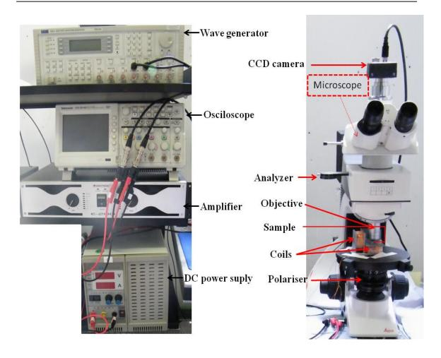
Fig 6.3: Picture of experimental set up
