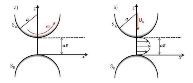
*Figure 3.2:* Scheme of the shear (a)) and the squeeze (b)) flow of two spheres of the same radius a. Here  $\varepsilon$  is the dimensionless gap parameter. This scheme has been redrawn from Ref. [82].
