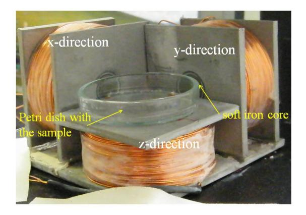
Fig 6.1: a) Picture of the arrangement of the three perpendicularly orientated solenoid coils with the soft iron core and
