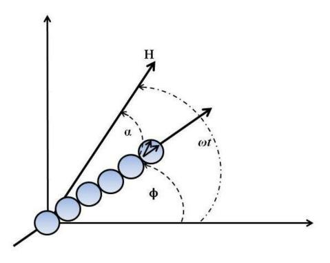
Figure 3.1: Chain of paramagnetic particles in rotating magnetic field.
