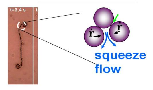
*Fig. 5.1.5:* Schematic draw of the area of the squeezing flow. One can see here that collapsing particles will squeeze out fluid remain between three interacting particles. Green arrow indicates Debye length (~10 nm) pointing that there is small gap between two particles.
