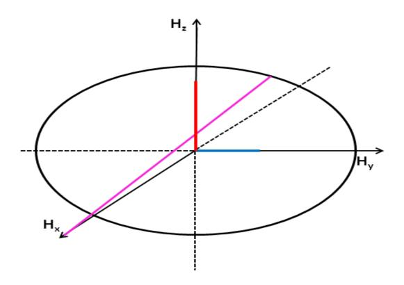
Fig 4.3: schematic representation of the elliptically polarized magnetic field is marked with the pink line, the red line represents field modulation in the direction of the z-axis and the blue line represents field modulation in the direction of the y-axis.
