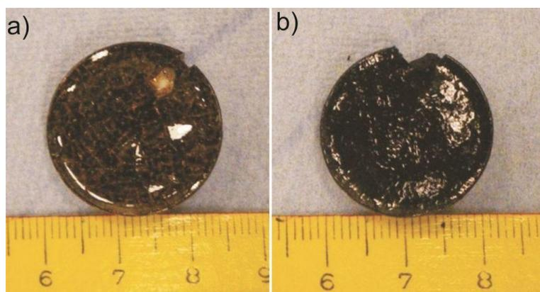
**Figure 1.** Pictorial presentation of Ni-131 (2 wt% nickel complex) before (a) and after pyrolysis at 600 °C for 2 hours (b).
