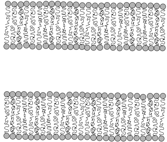
Figure 1.3: Sketch of a lyotropic liquid crystal in the L_\alpha phase. The space between the lamellae is filled with solvent (water).
