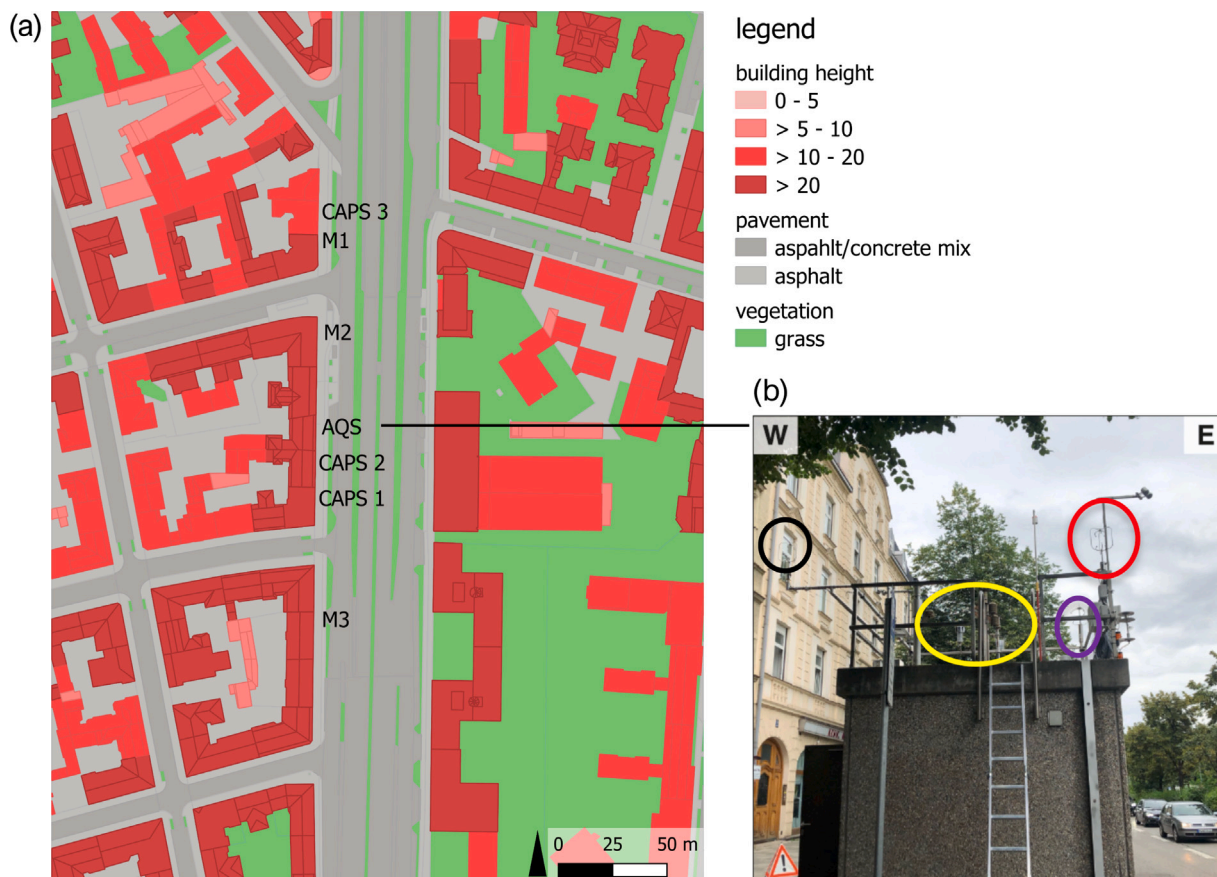
Fig. 2. (a) Closeup of the spatial distribution of the study area and its locations of measurements. The schematic pictures the exact area and land cover of the LES child domain of the study site consisting of an 8 lane street canyon of approx. 50 m width and buildings of 20 m height. M1 - M3 represent the alternating meteorological mobile measurement locations, CAPS 1–3 represent the alternating chemical measurement locations. (b) measurement devices of ultrasonic anemometer for roadside (red), windspeed, wind direction and temperature (purple), ultrasonic anemometer for pedestrian lane (black), mean NO 2 concentration (yellow).
