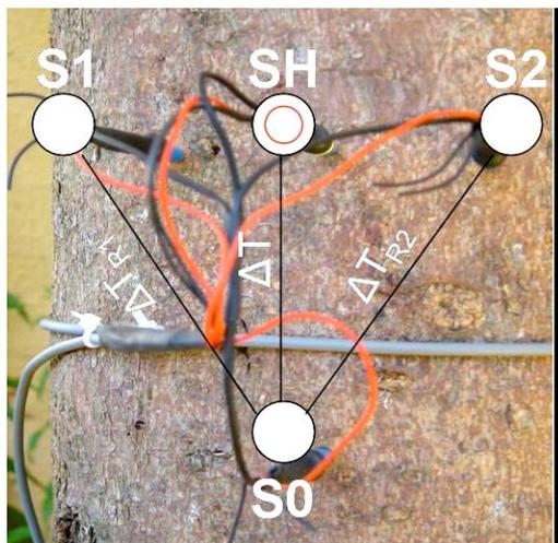
Plate 2. SF-L heat dissipation sensors installed into a tree. The probe SH was heated with a constant current power supply while SO, S1 and S2 were not heated. Wiring was done to measure temperature difference between SO-S1, SO-SH and SO-S2, where SO-S1 and SO-S2 are temperature differences due to natural temperature gradients on both sides of SH while SO-SH is due to sap flux.
