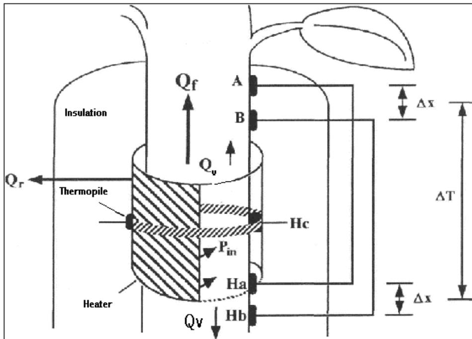
Figure 8. A schematic representation of a branch sensor (SHB method), showing arrangement of the thermocouples around the investigated stem as described in the text. Ha, Hb and Hc represent the respective temperature differences recorded at the logger
