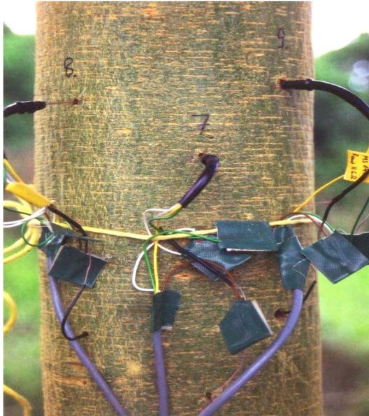
Plate 1. Three sap flow sensors numbered 7, 8 and 9, installed at different depths (0-20, 20-40 40-60 mm respectively) into the trunk of *A. xanthophloea*.
