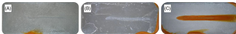
FIGURE 7 Optical images of scratched samples coated with system Z2 on steel 1.7335 treated at (A) 300°C, (B) 400°C, and (C) 500°C for 1 h in air and corroded in 5 wt.% NaCl solution for 504 h.
