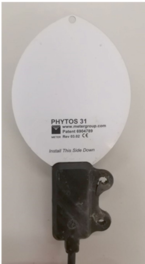
Fig. 3.17 Two different design examples of leaf wetness sensors: a type Campbell Scientific and b type Phytos 31, METER. Photos Eitzinger, BOKU
