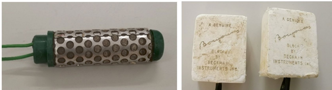
Fig. 3.20 Soil water potential sensors for agrometeorological use: a Watermark sensor (special granular matrix), Irrrometer Company Inc.; b Gypsum blocks, Beckman Instruments Inc. (all photos: Eitzinger, BOKU)
