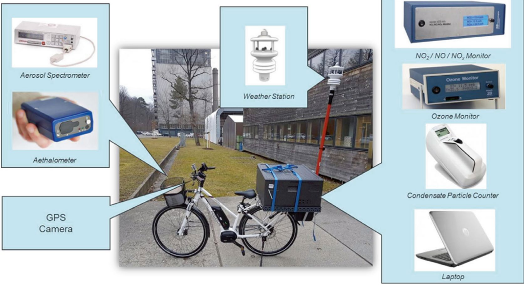
Fig. 2.10 Mobile measurements using a bicycle platform named MOBAIR. From Samad and Vogt (2020), © Authors CC BY 4.0. Note The weather station must be orientated vertically for wind measurements
