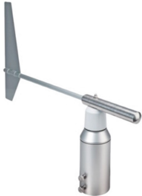
■ Fig. 3.12 Mechanical wind vane. Photo © Adolf Thies GmbH & Co. KG, Göttingen, Germany
