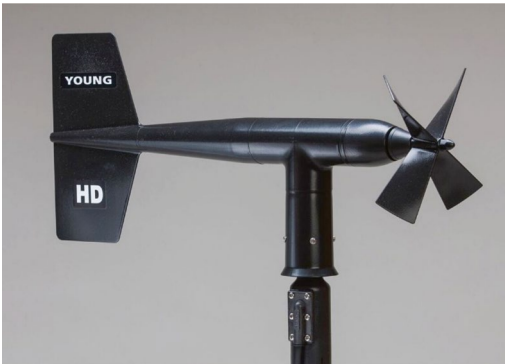
■ Fig. 3.13 Combination of propeller anemometer and mechanical wind vane, also called skyvane. Photo © R. M. YOUNG Company/GWU-Umwelttechnik GmbH, Erfstadt, Germany
