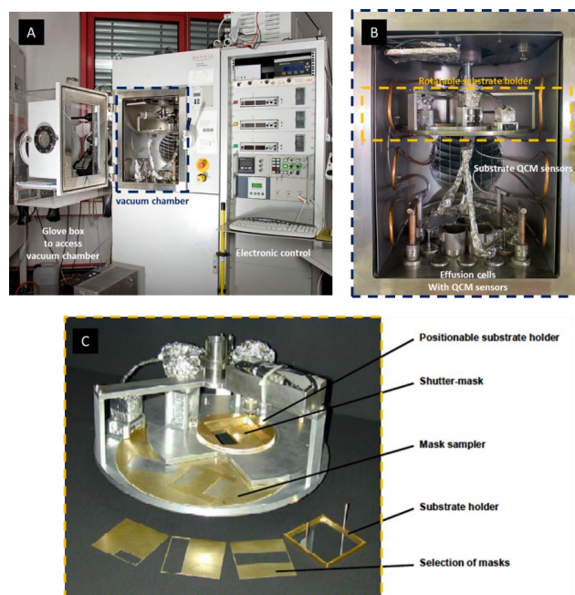
Figure 2. PVD setup in the Macromolecular Chemistry I at the University of Bayreuth. A) The setup consists of a vacuum chamber (framed in dashed blue lines) that is attached to a glovebox and an electronic control unit. B) The vacuum chamber is equipped with three effusion cells, that are all equipped with a QCM sensor, additionally two QCM sensors in the close proximity to the substrate and a rotatable substrate holder (framed in dashed orange lines). C) The rotatable substrate holder consists of a positionable substrate holder that can be turned in 90° increments during operation, a shutter mask, and a mask sampler. Source: University of Bayreuth, Macromolecular Chemistry I.
