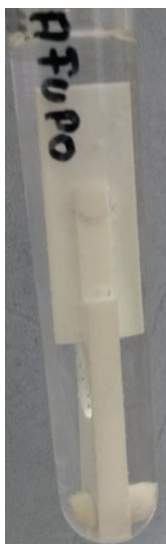
Fig. 91 Schlenk tube with a home-made PTFE magnetic stirring bar extension paddle used for the syntheses of PFEG3ES-FRP-UP and PFEG3ES-RAFT-UP.
