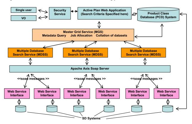
Figure 3 – COVITE flow architecture diagram
