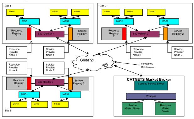
Figure 4 – Cat-COVITE architecture – centralised use case
