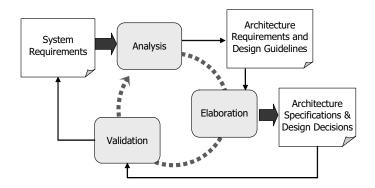
Figure A.1. The Architecture Design Process
