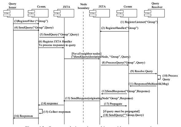
Figure 15 - Query resolution using multicast with response service
