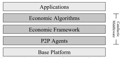
Figure 2 - A layered architecture for resource allocation
