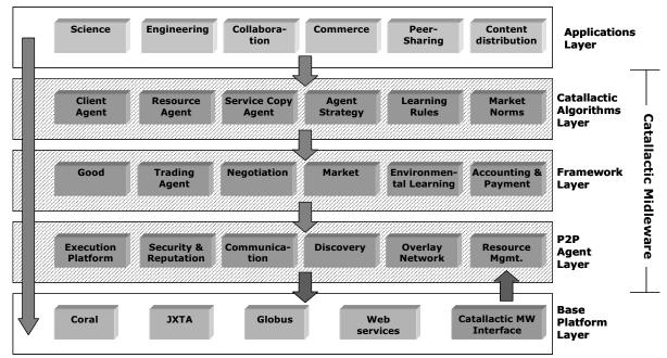
Figure 9 - CATNETS architecture – Layered View
