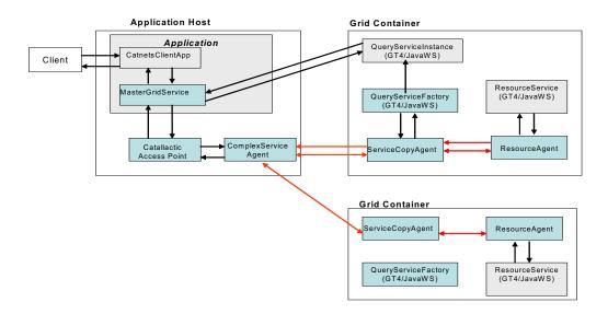
Figure 18 – Physical deployment of application and middleware components
