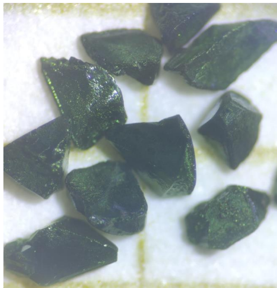
Figure S25. Microscopic images of [\text{Spiro-MeOTAD}]^+[\text{Cu}^{\text{I}}(\text{TFSI})_2]^- crystals before the hexane washing step. Lines in the background are 2 mm by 1 mm.
