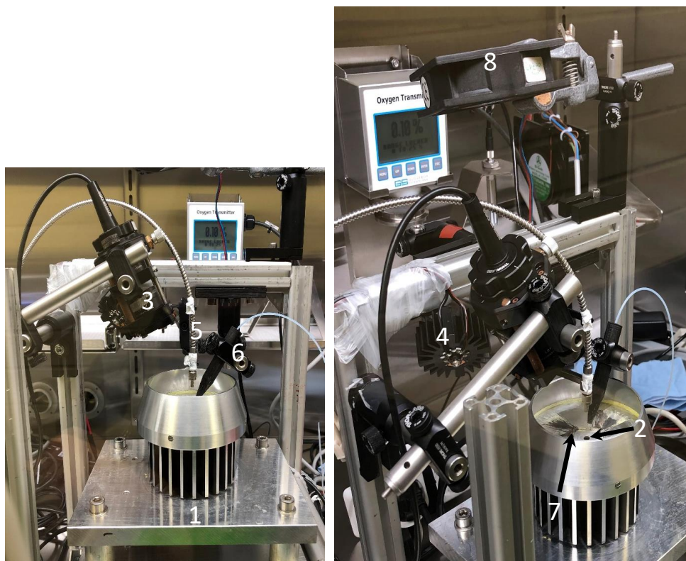
Fig. S1: Photographs of the setup used for measuring the in situ optical data during spin coating.
