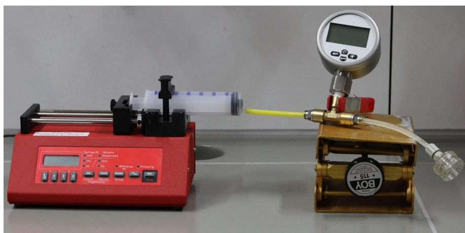
Figure S7. Measurement setup for the aqueous filtration of PS microparticles from water with parallel measurement of the pressure drop.
